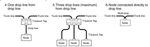
Various forms of connection can be used on the same Network, as shown in the following diagram. Any number of nodes up to 63 can be connected onto a single drop line.
